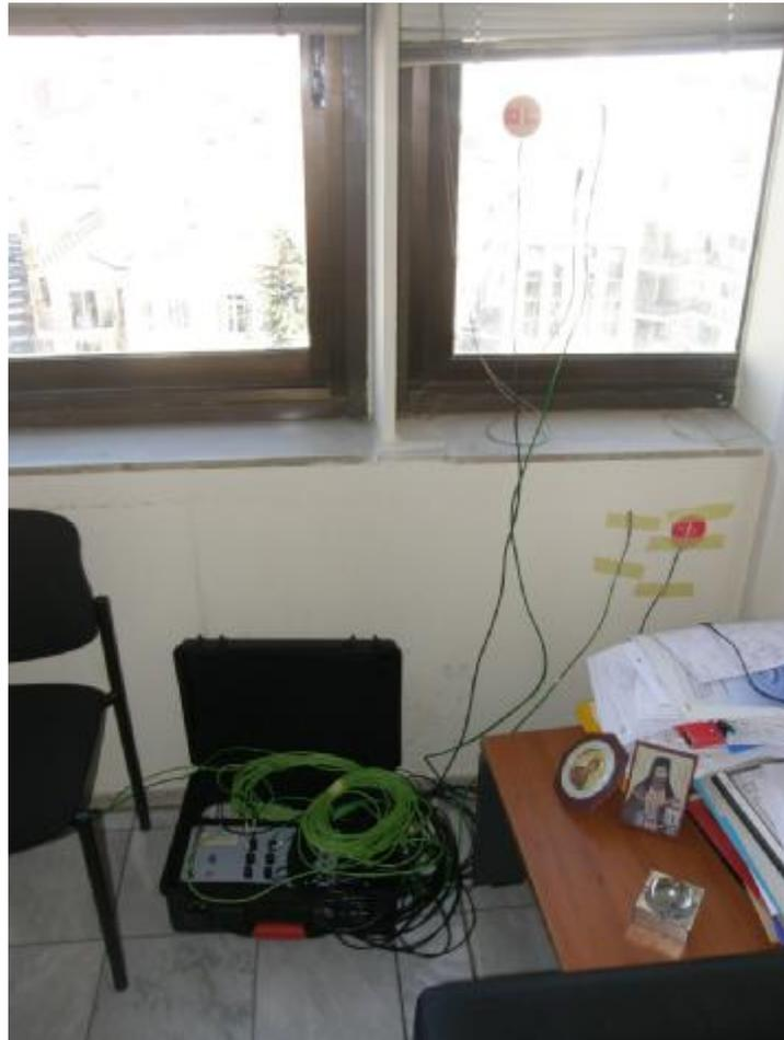
The duration of the measurement was 72 hours - one measurement was carried out on the opaque structural element (wall), while the second one concerned the transparent structural element (window).
