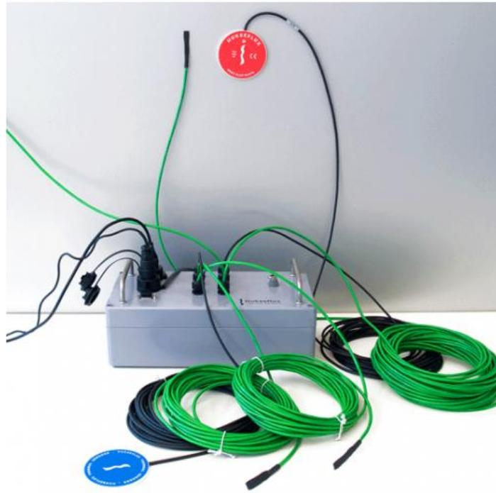
The TRSYS01 is a tool for measuring and analyzing the thermal resistance of building materials with the measurement made in existing buildings. It can be used for measurements in accordance with ISO 9869 and ASTM C1155 / C1046.
